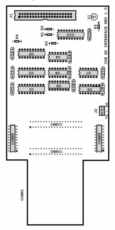
The PCB has one set of jumpers, J2, used to select the addresses at which the device is active. The options are:
